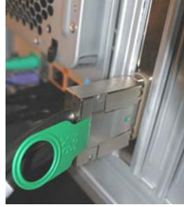
Connect x8 end to the host card.
